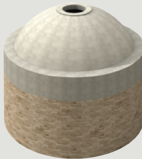
Hemispherical dome with oculus
